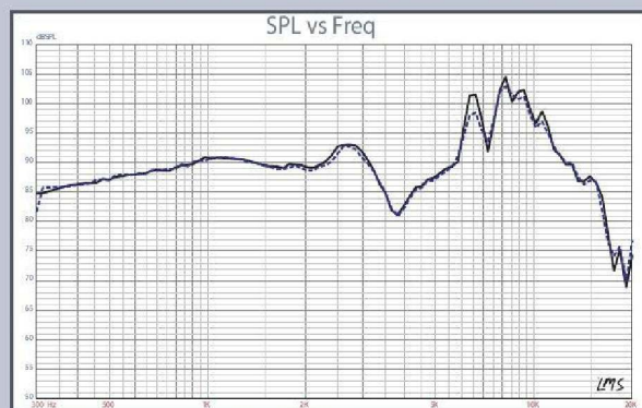
FIGURE 12: Scan-Speak 18WU4747T00 two-sample SPL comparison.
