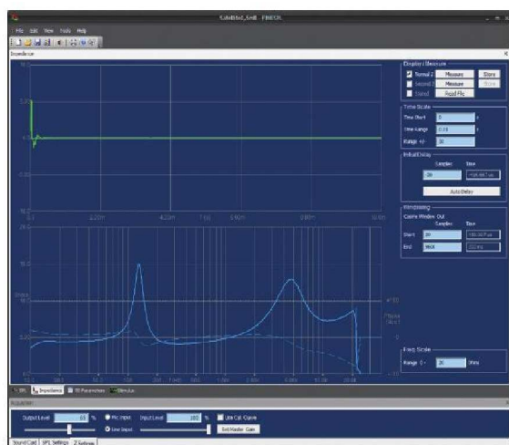
FIGURE 3: FINESPL impedance magnitude and phase graph.
