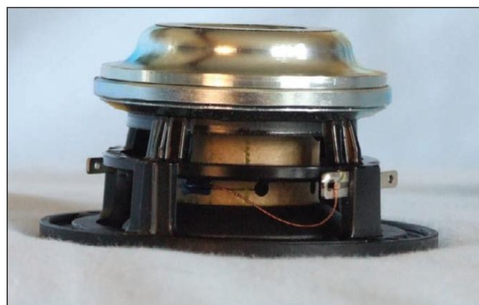
Photo 4: A neodymium motor with a neodymium ring magnet and a polished milled return cup drives the 5F/8422T01's cone assembly.
