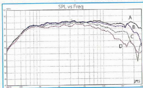
FIGURE 19: D2004/602000 horizontal on- and off-axis frequency response (A = 0°; B = 15°; C = 30°; D = 45°).
