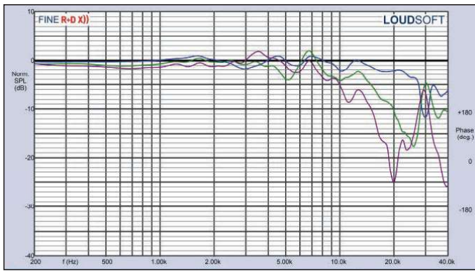
Figure 5: Scan-Speak D2010/852100 normalized on- and off-axis frequency response (0° = black; 15° = blue; 30° = green; 45° = purple)
