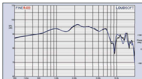
Figure 26: Scan-Speak Ellipticor 18WE/4542T00 midwoofer two-sample SPL comparison
