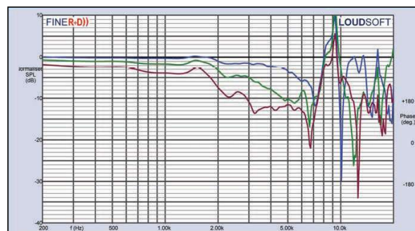
Figure 24: Scan-Speak Ellipticor 18WE/4542T00 normalized on- and off-axis frequency response (0° = black; 15° = blue; 30° = green; 45° = purple)
