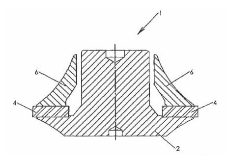
This concept is part of a quest to design an ultra linear motor system. It is possible to make linear systems with traditional over-hung magnet systems, but the under-hung principle can be realized with an overall lower moving mass for the loudspeaker together with a lower inductance when combined with copper caps.
