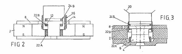
The original SD concept is based on an electrically conductive extended cap (typically copper), as described and patented by Ragnar Lian, 1972, then working at Scan-Speak, and presented in AES papers in 1974 and 1988. Prior to this a copper cap had been used by others, e.g. Philips.
